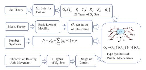
Fig. 2. Type design procedures of parallel robotic mechanisms
